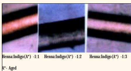
Fig. 6 : Microscopical observation of the effect of modifier (1% ferric chloride) on colour modification with henna and indigo
