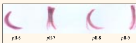
Fig. 3: Effect of pH on colour produced with henna and indigo
