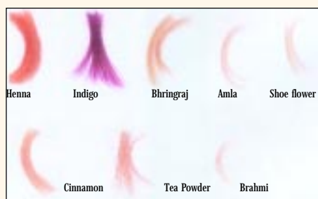
Fig. 1 : The different colours produced by grey hair (white) after treatment with different herbal powders in the form of paste
