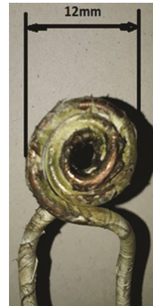
Fig. 3 — Induction heating coil having 12 mm diameter
