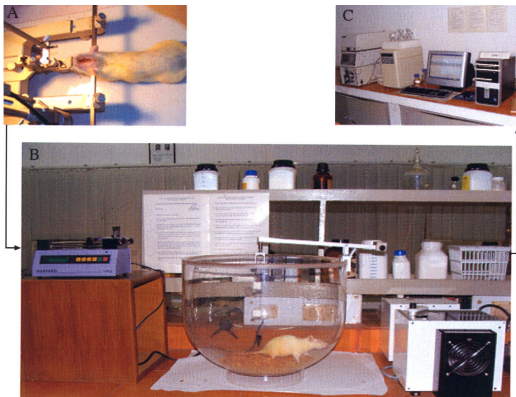
Fig. 1— In vivo microdialysis setup for the collection of extracellular fluid from rat striatum. (A) - Stereotaxic apparatus for probe implantation; (B) - In vivo microdialysis set up; and (C) - HPLC/ECS detection system.
