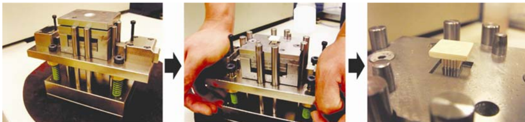
Fig. 2-Schematic diagram of the procedure of sample separation from the inner block by using an ejecting jig
