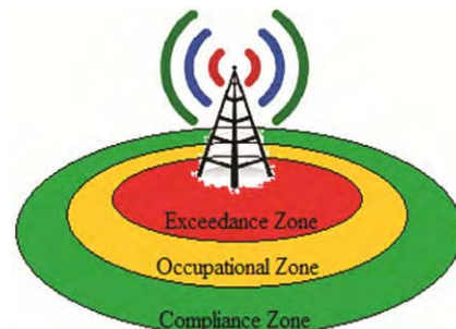
Fig. 2 — Marking of different zones around a base station antenna
