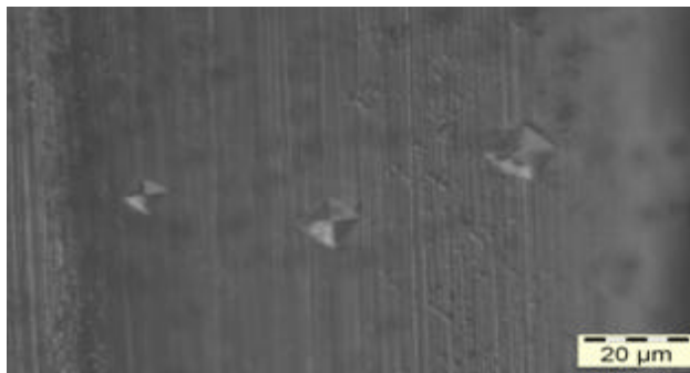
Fig. 4—SEM photograph of coated section with microhardness indentations
