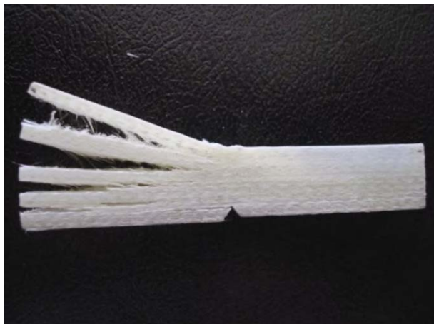
Fig. 12—Failure of a glass-epoxy specimen with side-on oriented notch at low temperature
