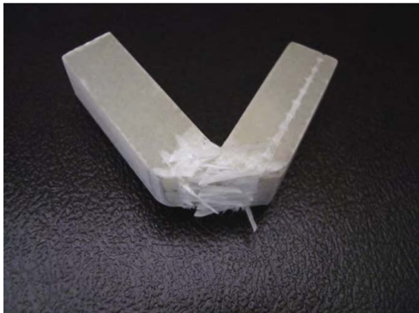
Fig. 11—Failure of a glass-epoxy specimen with edge-on oriented notch at room temperature
