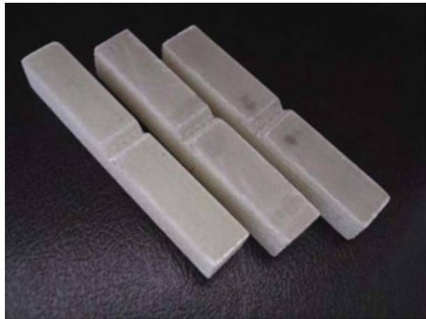
Fig. 3—Samples of fabricated specimens for Charpy impact test
