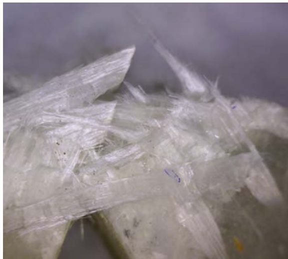
Fig. 15—Microscopic examination of fractured specimen with edge-on notch orientation after one day exposure at -30^{\circ}\text{C}
