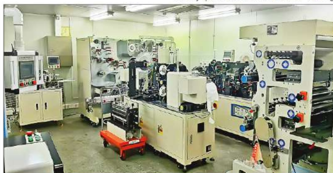
Assembly Line Equipments Inside 1% RH Dry Room for Making 1000 cells/day
