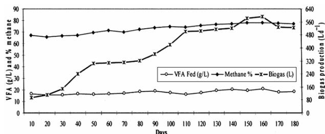
Fig. 2—Profile of VFA fed, biogas production and methane content in MRs
