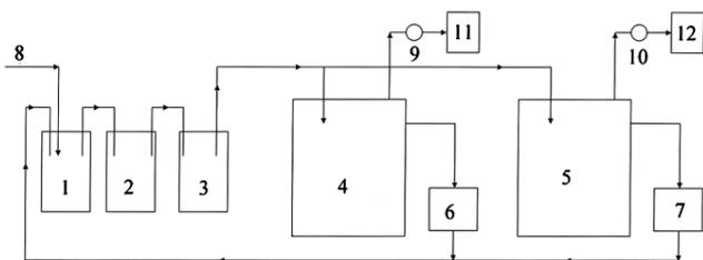
Fig. 1—Schematic presentation for biphasic biomethanation of spoiled mango puree: 1, AR1; 2, AR2; 3, AR3; 4, MR1; 5, MR2; 6 & 7, MRDCT; 8, Spoiled mango puree; 9 & 10: Gas flow meter; and 11 & 12, Gas holders.
