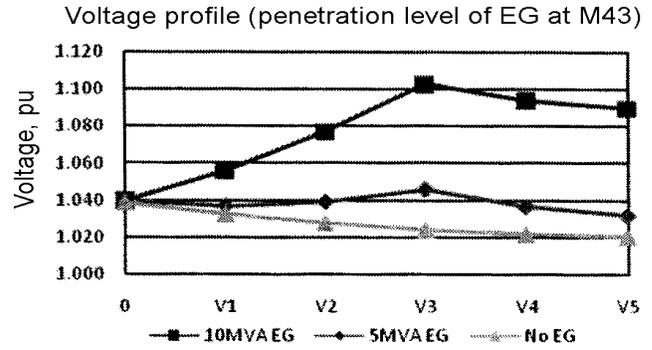
Fig. 6—Feeder 4 voltage profile with various rating of EGs at  $M_{43-MBB}$
