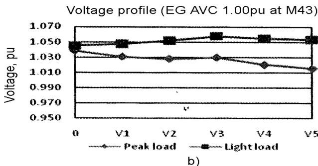
Fig. 5—Feeder 4 voltage profile with EG terminal voltage at: a) 1.00 pu; b) 1.03 pu
