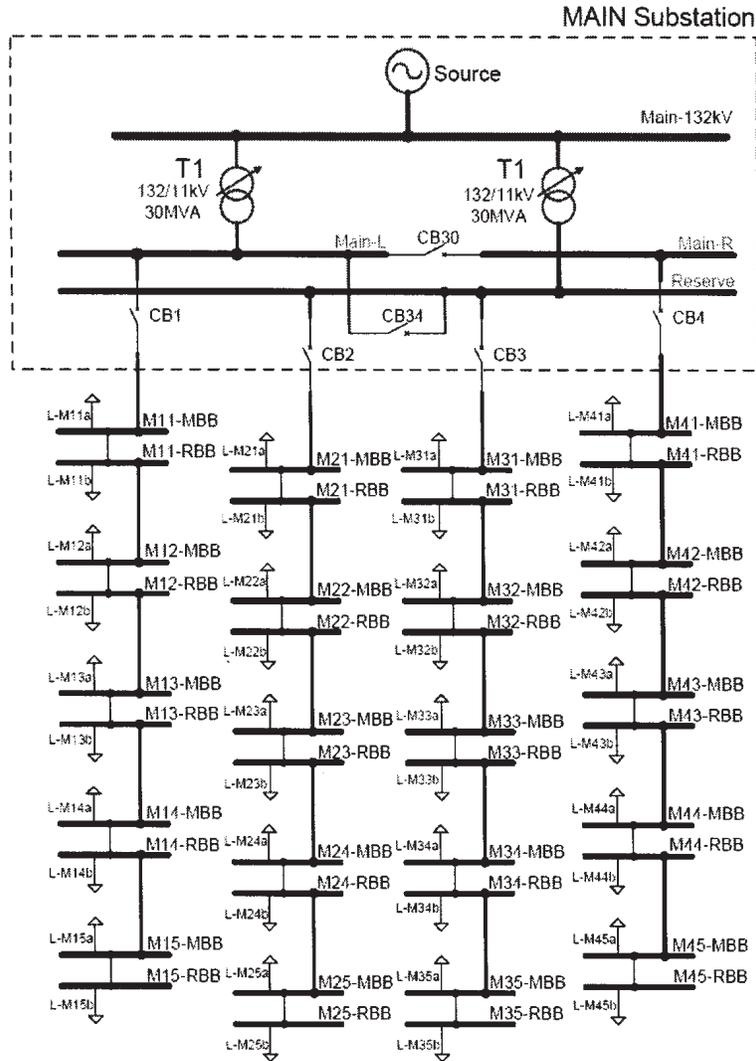
Fig. 1—Single line diagram of generic distribution network
