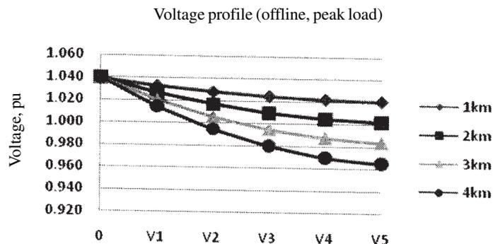
Fig. 2—Network voltage profile with Main substation voltage at 1.05 pu
