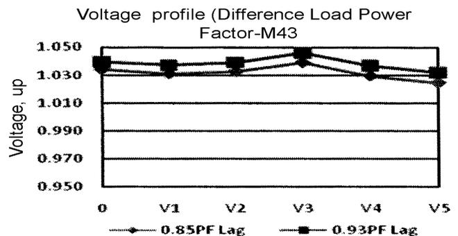
Fig. 8—Feeder 4 voltage profile with EG at  $M_{43-MBB}$  with different network power factor
