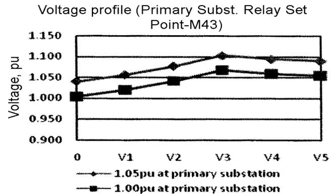
Fig. 7—Feeder 4 voltage profile with MAIN substation voltage at 1.00 pu and 1.05 pu
