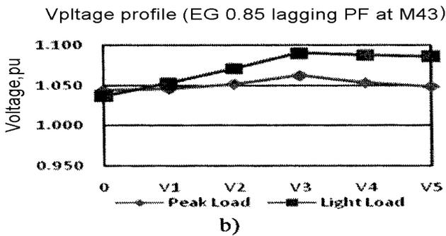
Fig. 4—Feeder 4 voltage profile with EG operating at: a) 0.85 leading power factor; and b) 0.85 lagging power factor
