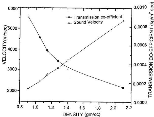
Fig. 2 — Variation in sound velocity and transmission coefficient as a function of density in plastics
