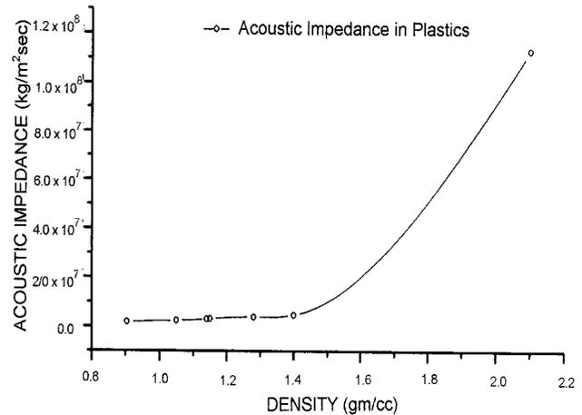
Fig. 3 — Variation in acoustic impedance as a function of density in plastics
