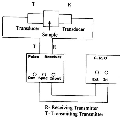
Fig. 1 — Block diagram of ultrasonic system for velocity measurement of solid samples
