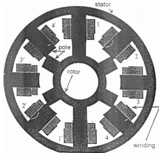
Fig. 1a — Cross-section of 4-phase SRM
