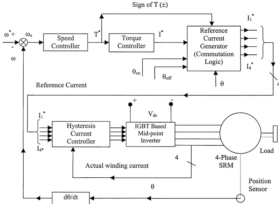
Fig. 3 — Block diagram of SRM drive system with PID speed controller
