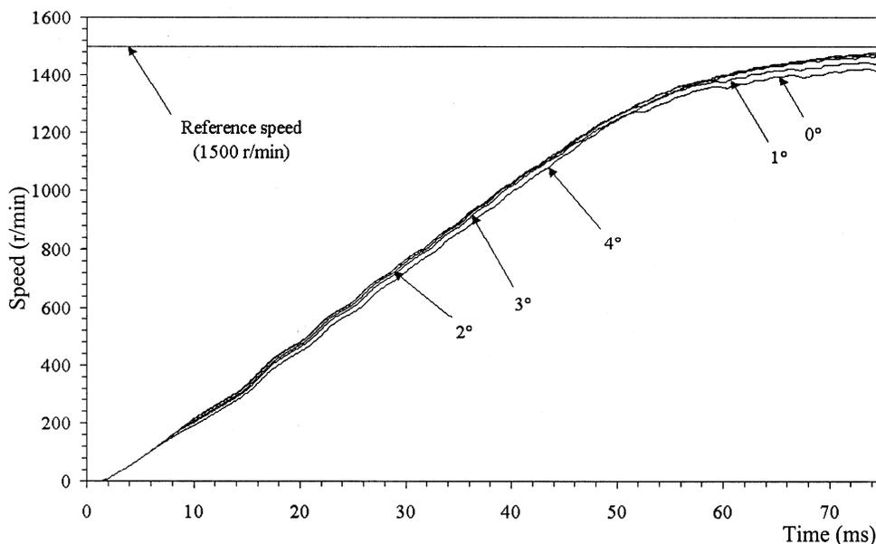
Fig. 4a — Full-load starting speed response of SRM with  $12^\circ$  turn-on angle and different turn-off angles, when speed controller is out of service
