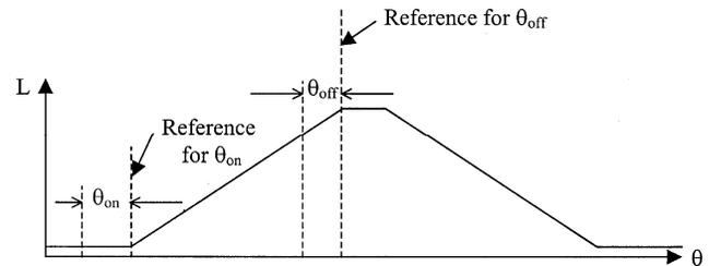
Fig. 2c — Turn-on and turn-off angles of any one phase of SRM
