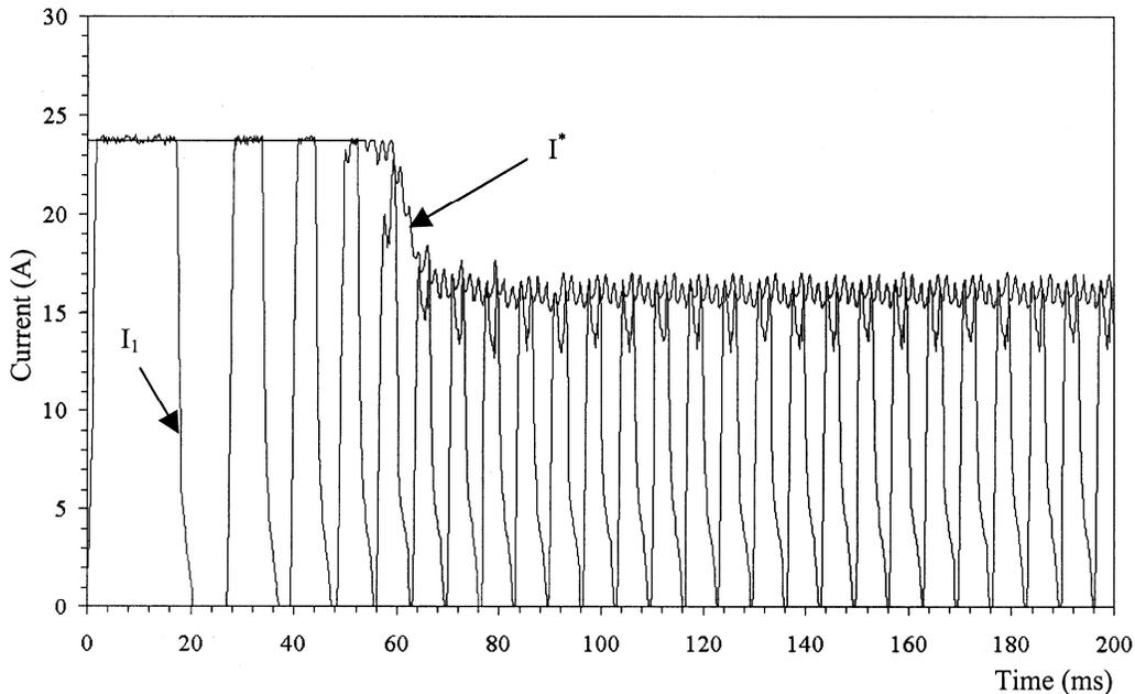
Fig. 9a — Phase-1 current response of SRM with optimum pair ( $13^\circ$ ,  $3^\circ$ ) of switching angles during full-load starting, when PID speed controller is in service
