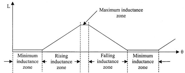
Fig. 2b — Different zones of inductance of any one phase of SRM
