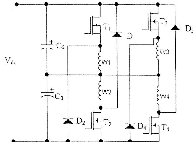
Fig. 1b — Mid-point inverter for SRM
