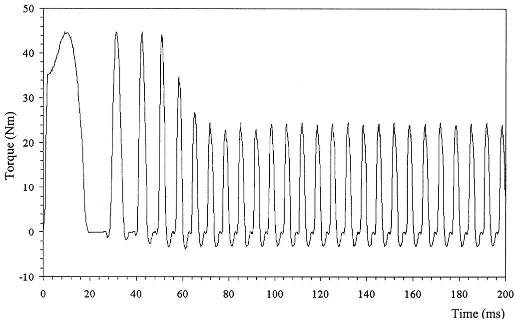
Fig. 9b — Phase-1 torque response of SRM with optimum pair ( $13^\circ$ ,  $3^\circ$ ) of switching angles during full-load starting, when PID speed controller is in service
