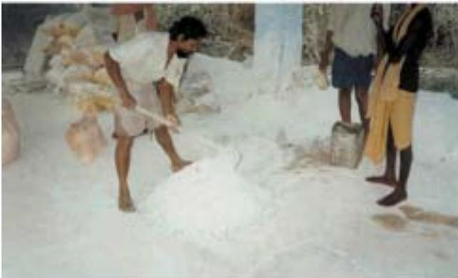
Fig.5 Slaking of powder lime
