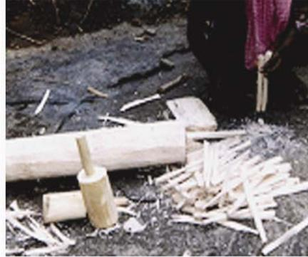
Fig.3 Making splinters
