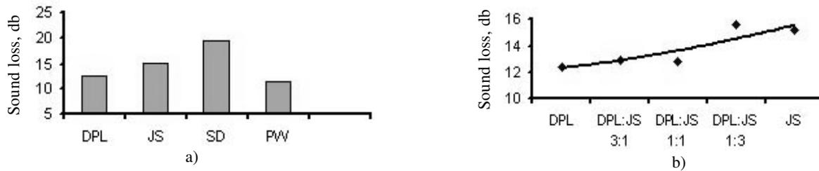
Fig. 3—Sound insulation: a) Particle boards; b) Effect of blending DPL with JS
