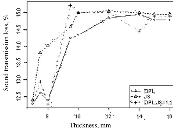
Fig. 5—Scatter plot of sound loss of different type of board
