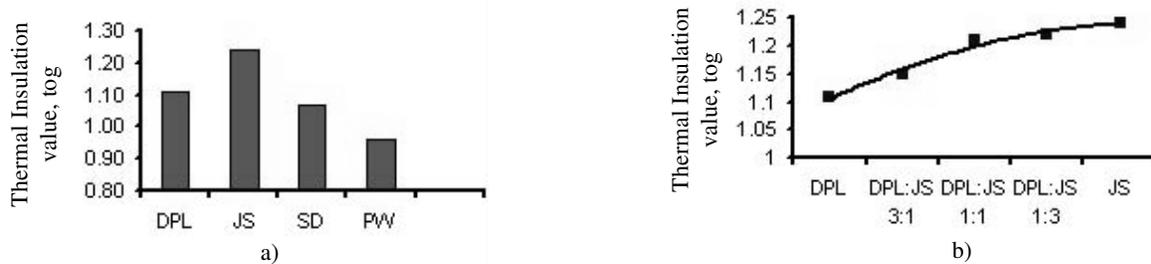
Fig. 4—Thermal Insulation: a) Particle boards; b) Effect of blending DPL with JS
