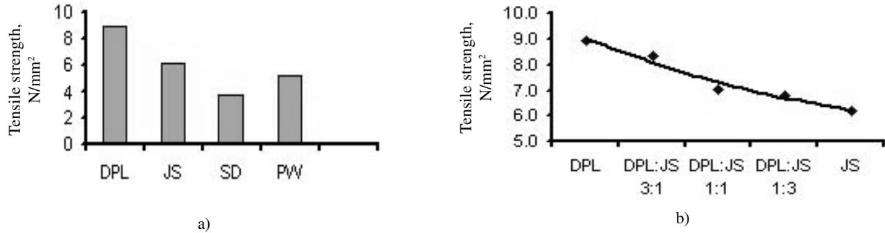
Fig. 1—Tensile strength: a) Particle boards; b) Effect of blending DPL with JS
