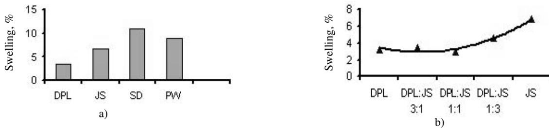
Fig. 6—Swelling: a) Particle boards; b) Effect of blending DPL with JS
