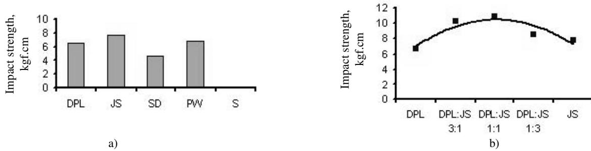
Fig. 2—Impact strength: a) Particle boards; b) Effect of blending DPL with JS
