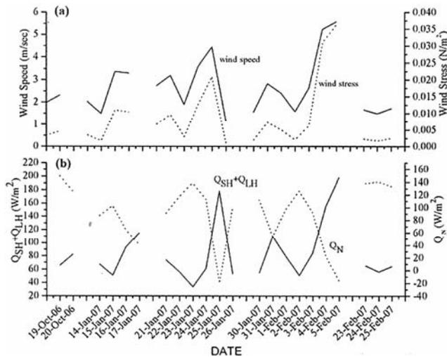
Fig. 7—Daily mean variability of: (a) wind speed (m/sec) and wind stress ( $\tau$ , N/m<sup>2</sup>); (b) Net heat flux (Q<sub>N</sub>, W/m<sup>2</sup>) and enthalpy (Q<sub>SH</sub>+Q<sub>LH</sub>, W/m<sup>2</sup>)
