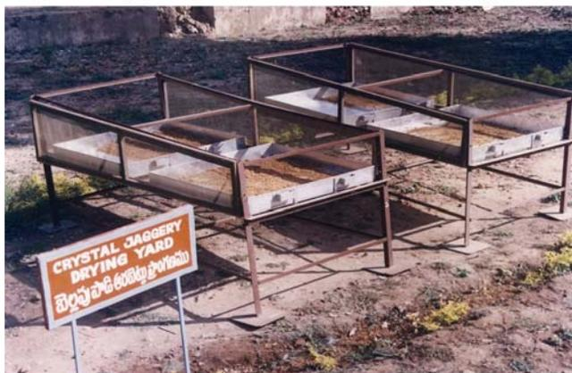
Fig.14 Drying of granular jaggery
