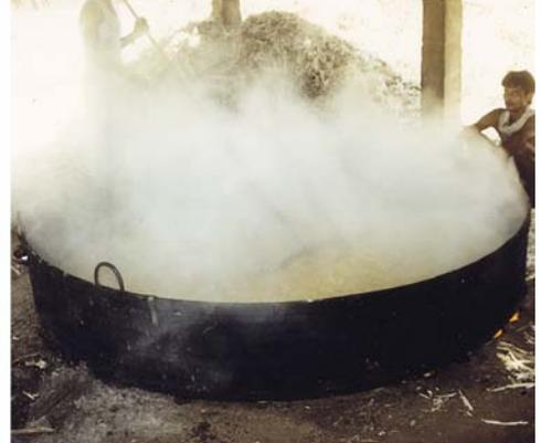
Fig. 7. Juice boiling in open pan
