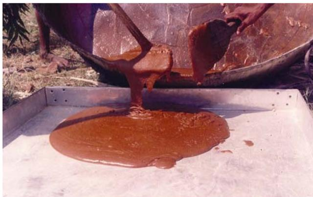
Fig.12 Hot thick syrup transferred to tray for scrapping
