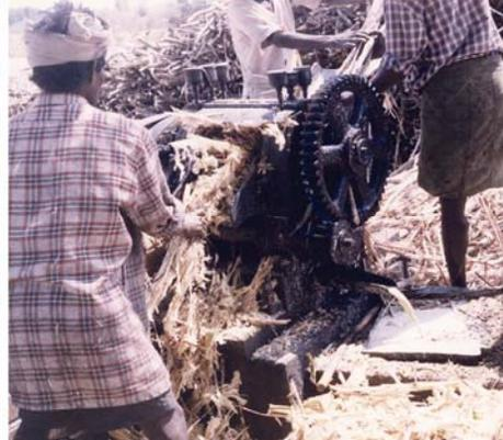
Fig. 6 Horizontal three roller crusher
