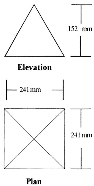
Fig. 1c Fiber Glass Pyramid (FGP1)
