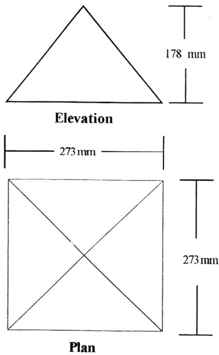
Fig. 1d Fiber Glass Pyramid (FGP2)
