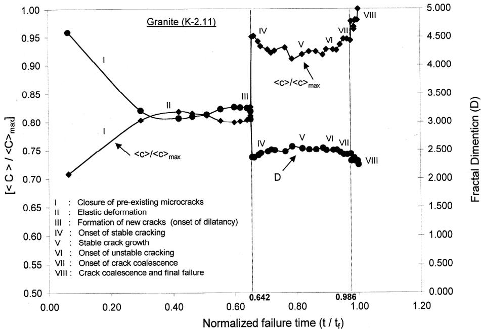
Fig. 4 — The inferred mean crack length (normalized) and observed fractal dimension ( $D=2b$ ) are plotted as a function of normalized failure time. Sharp changes in them were found to occur at the onset of dilatancy (stage III, i.e., at  $0.642 t_f$ ) and at the onset of crack coalescence (stage VII, i.e., at  $0.986 t_f$ ) as inferred from the AE data of a granite rock
