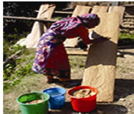
Fig. 10 Pasting the pulp on plank
