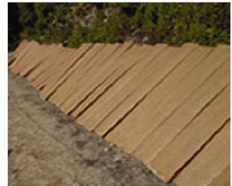
Fig. 11 Drying of pasted pulp
