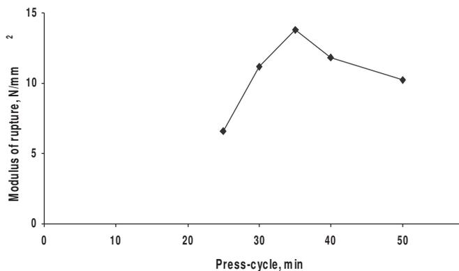
Fig.3—Effect of press-cycle on modulus of rupture of composite board
