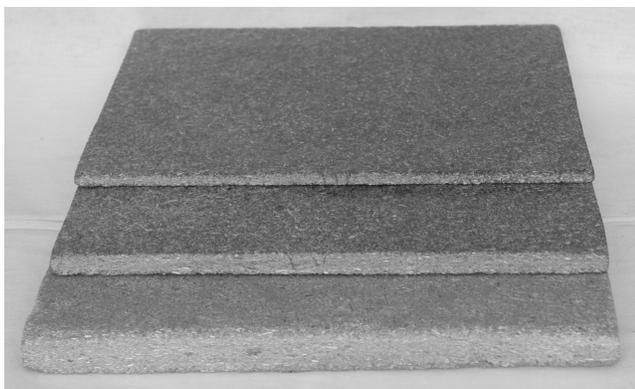
Fig. 6—Composite boards of varying thickness [ 7 mm, 12 mm & 20 mm (from top) ] using sticklac
