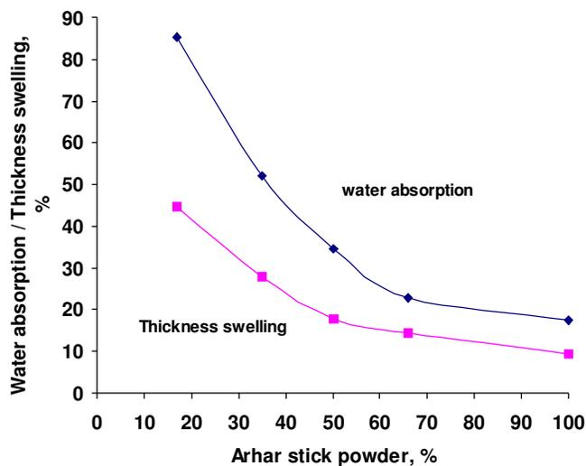
Fig.5—Influence of particle size on water absorption and thickness swelling of composite board
