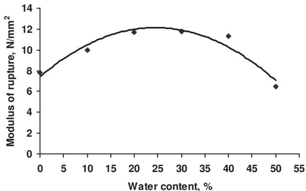
Fig. 2—Effect of water content of mat to be hot pressed on modulus of rupture of composite board using sticklac in aqueous medium
