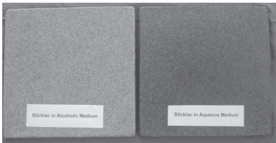
Fig.1—Composite board from *arhar* stick using sticklac in alcoholic and aqueous medium respectively
