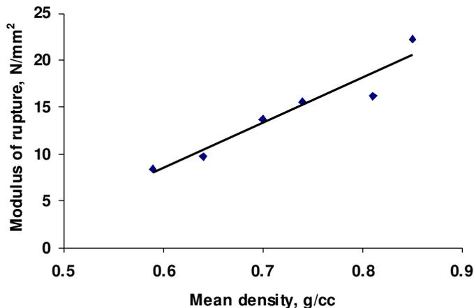
Fig.4—Change in modulus of rupture with density of composite board
