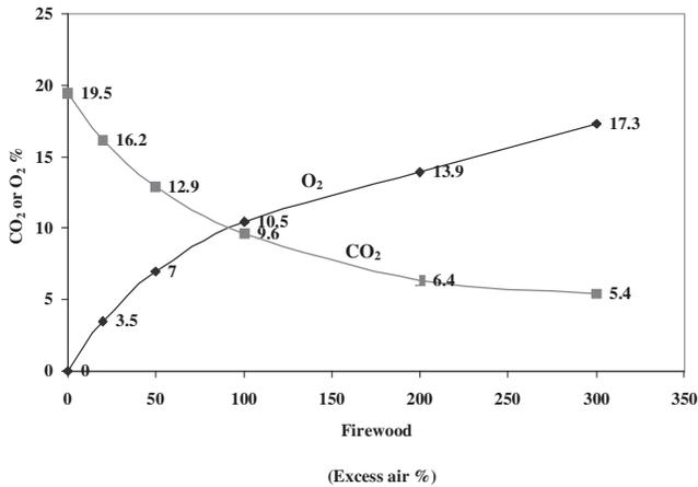
Fig. 1—CO<sub>2</sub>% / O<sub>2</sub>% vs excess air curve for firewood
