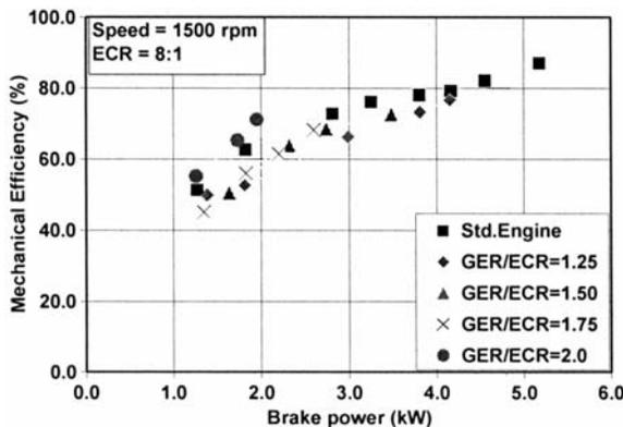
Fig. 4— Variation of mechanical efficiency with brake power
