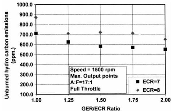
Fig. 7— Variation of unburned hydrocarbons emissions with GER/ECR ratio at maximum output points
