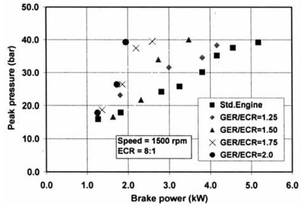
Fig. 5— Variation of peak pressure with brake power output
