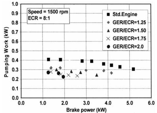
Fig. 6— Variation of pumping power with brake power output
