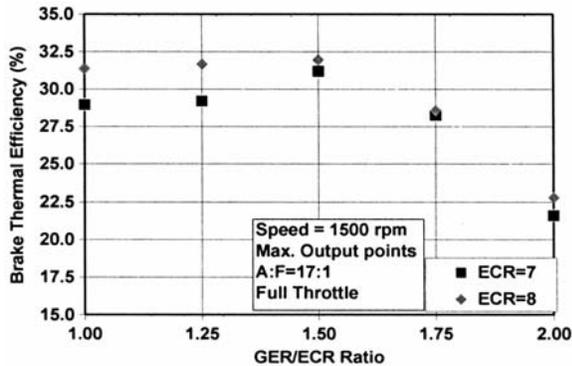
Fig. 3— Variation of brake thermal efficiency with GER/ECR ratio at maximum output points
