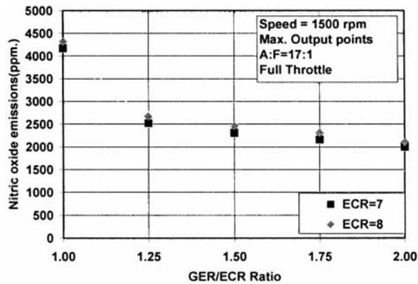
Fig. 8— Variation of nitric oxide emissions with GER/ECR ratio at maximum output points
