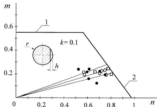
Fig. 5—Diagram of shakedown of studs with crack: (O) M48×3; (■) M48×4; (□) M48×5 (chromium steel); (●) M48×4 (high temperature steel)
