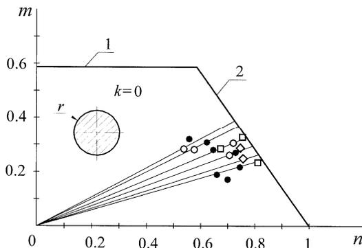
Fig. 4—Diagram of shakedown of studs without crack: (O) M48×3; (■) M48×4; (□) M48×5 (chromium steel); (●) M48×4 (high temperature steel)
