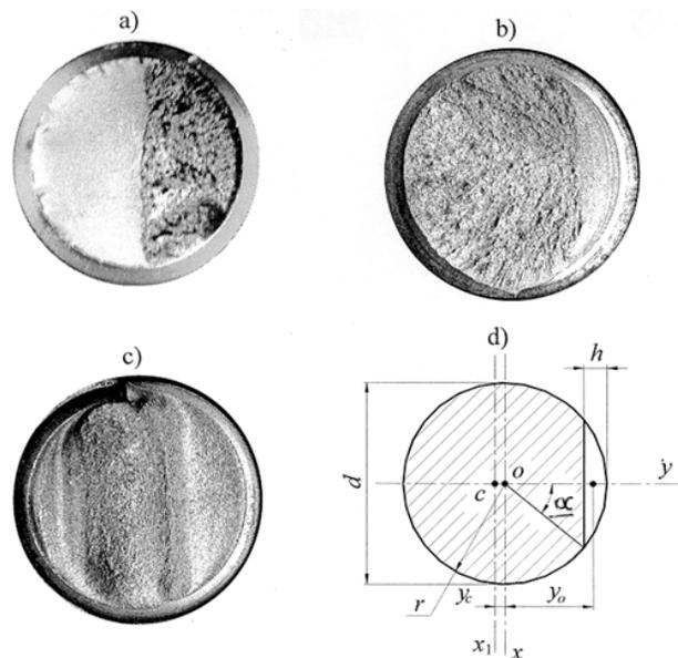
Fig. 3—The breaks view of a stud-bolt with crack: (a) and (b) crack is on one side of stud; (c) crack is on two side of stud; (d) model of cross-section
