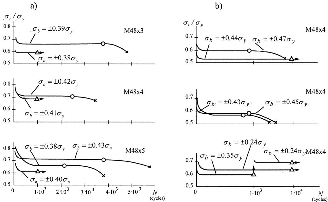
Fig. 2—Change in tightening of threaded joints made of chromium steel (a) and of high temperature steel (b): (O) threshold; ( $\Delta$ )→ test is terminated; (x) full fracture, ( $\uparrow$ ) overprestress,
