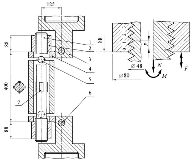
Fig. 1—Stud-nut bending equipment and stud-nut position (system of reading and crack initiation): (1) stud, (2) nut, (3) holder, (4) lever; (5) roller, (6) axis and (7) strain gage
