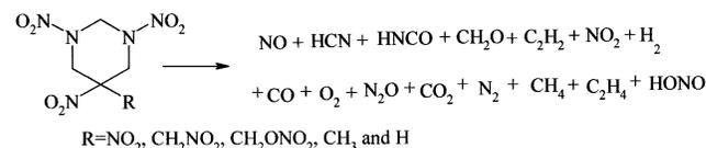
They observed that the substitution of groups at the 5<sup>th</sup> position of TNP have major influence on the decomposition of most of these molecules. TG data obtained during this work suggests that the major decomposition step shifted to higher temperature on insertion of methyl group (**10**) at 5<sup>th</sup> position in TNP whereas introduction of nitro (**4**), nitratomethyl (**8**) and azidomethyl (**7**) at this position resulted in the shift to lower temperature.
