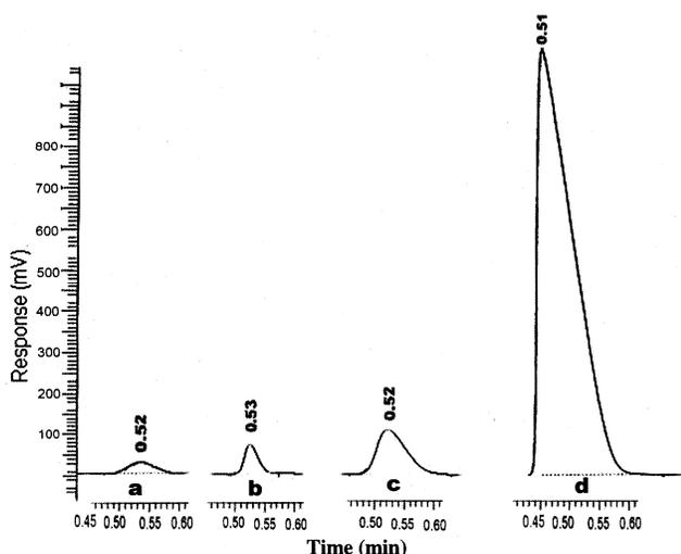
Fig. 1—Mineralization of high concentration of PNP (2.143 mM) on the basis of emergence of CO<sub>2</sub> peak detected by GC analyzer at a (10 h, 84935  $\mu$ V.s), b (20 h, 218860  $\mu$ V.s), c (30 h, 324091  $\mu$ V.s) and d (standard CO<sub>2</sub>, 10325786  $\mu$ V.s).
