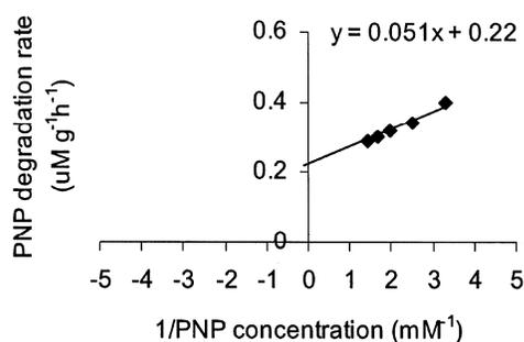
Fig. 5—Lineweaver-Burk plot of PNP degradation as a function of concentration for evaluating rate constant of PNP degradation by *P. putida*.
