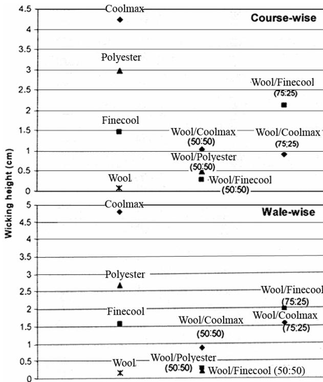
Fig. 7 – Influence of type of fibre at the end of 1<sup>st</sup> min in the vertical wicking
