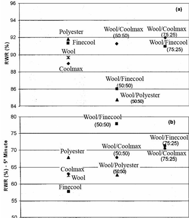
Fig. 8 – Influence of type of fibre at 5 min on the drying rate [(a) standard conditions, and (b) 33°C temperature]
