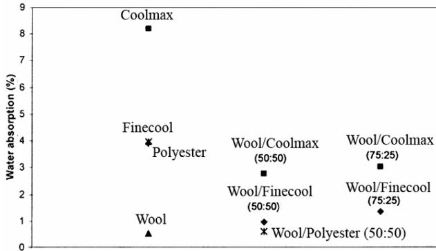
Fig. 6 – Influence of type of fibre at the end of 1<sup>st</sup> min in the horizontal wicking
