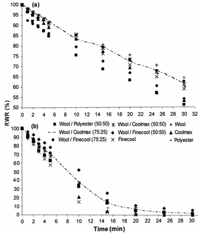
Fig. 5 – Drying rate (a) at standard conditions, and (b) at 33°C temperature
