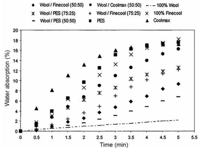
Fig. 3 – Horizontal wicking curve
