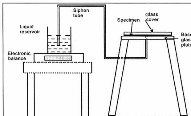
Fig. 2 – Horizontal wicking apparatus
