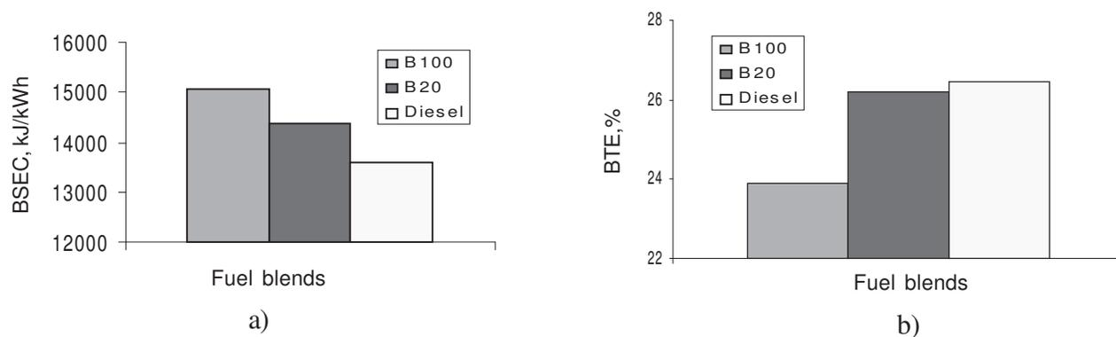
Fig. 2—Engine performance at full load: a) BSFC; b) BTE
