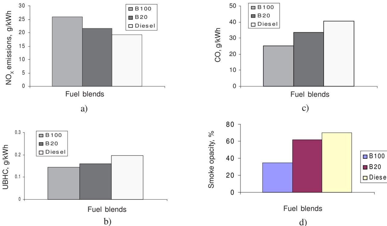
Fig. 3—Engine emissions at full load: a) NO<sub>x</sub>; b) UBHC; c) CO; d) smoke
