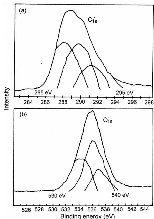
Fig. 3 — Binding energy (BE) of (a)  $\text{C}^*_{1s}$  of the 20% mercerized fiber; (b)  $\text{O}^*_{1s}$  of the 20% mercerized fiber
