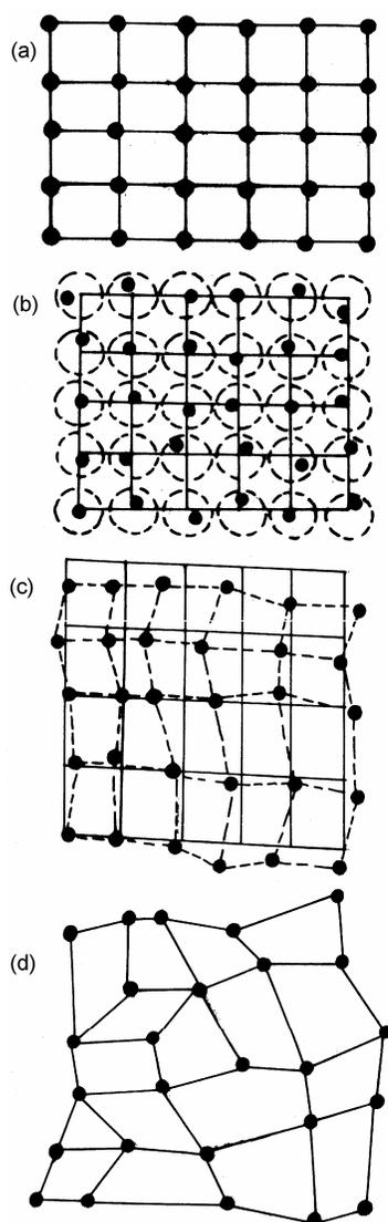
Fig. 1 — Lattice structures of cellulose (a) Perfect (undistorted) lattice, (b) Lattice distortions of the first kind, (c) Lattice distortions of the second kind and (d) Amorphous structure (no lattice)
