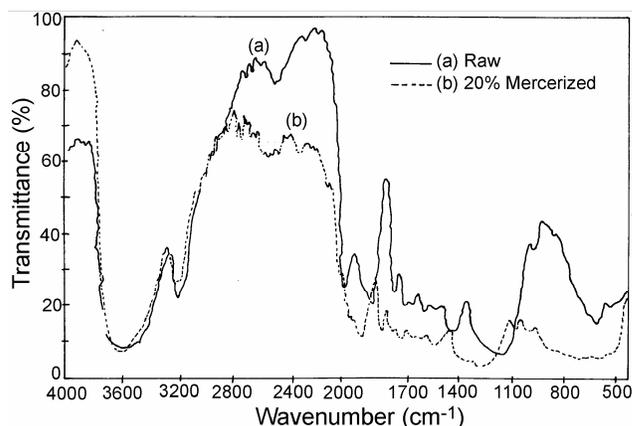
Fig. 4 — Overlapped IR spectra of the raw and 20% mercerized fiber
