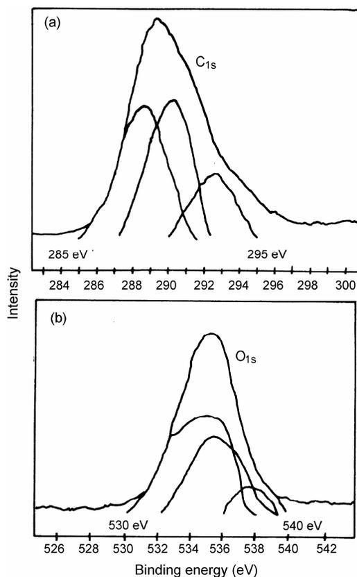
Fig. 2 — Binding energy (BE) of (a)  $\text{C}_{1s}$  of the raw fiber, (b)  $\text{O}_{1s}$  of the raw fiber
