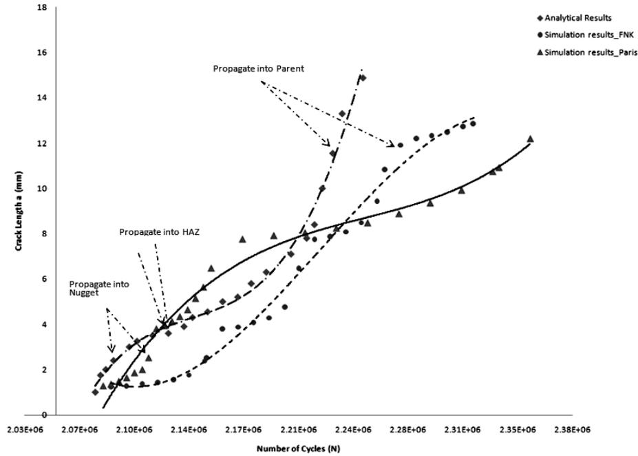
Fig. 8—Total crack length versus number of cycles for 270 MPa maximum applied stress with load ratio R= 0.1
