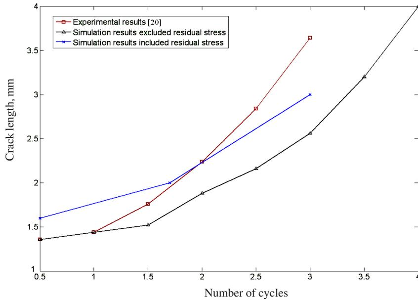
Fig. 9—Effect of residual stress on simulation result in comparison with experiment (Crack propagation under max. stress of 270 MPa and R= 0.1)
