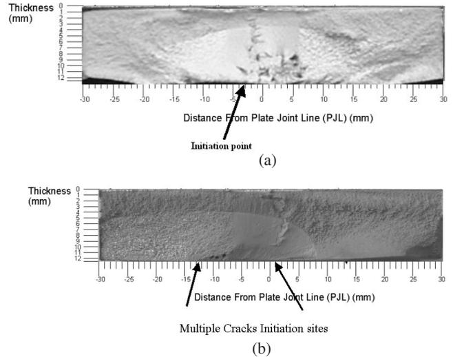
Fig. 2—Replication images for HCF of 2024-T351 Al Alloy FSW specimen: a) Polished mirror FSW joint under 270 MPa maximum applied stress with load ratio R= 0.1; and b) As welded FSW joint under 161 MPa maximum applied stress with load ratio R= 0.1
