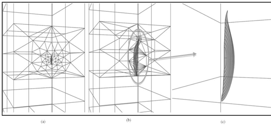
Fig. 6—Crack growth profile under  $\sigma=300$  Mpa: a) Initiation of 1 mm crack in specimen; b) Crack profile after 10 steps of propagation; and c) Crack starts to deviate from its original plane after 10 steps of propagation
