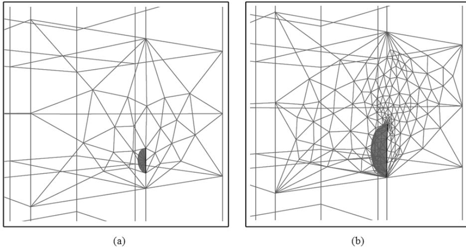
Fig. 5—Meshing distribution around crack tip: a) First step after initiation; and b) Remeshed area after 4 steps of propagation
