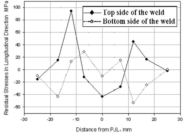
Fig. 4—Longitudinal residual stress distribution along FSW 2024-T351 Al alloy joint20
