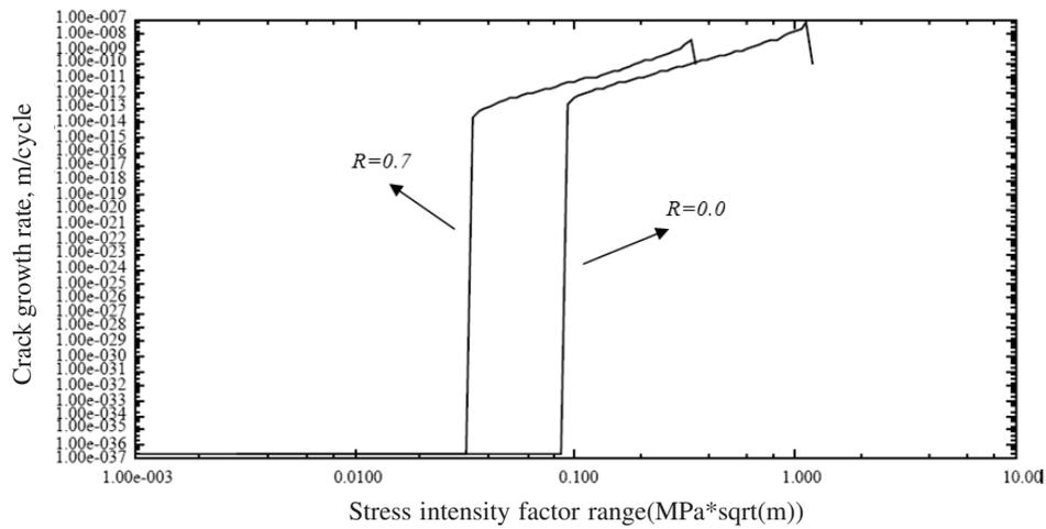
Fig. 7—Crack growth rate data for Al 2024-T351 with different load ratios
