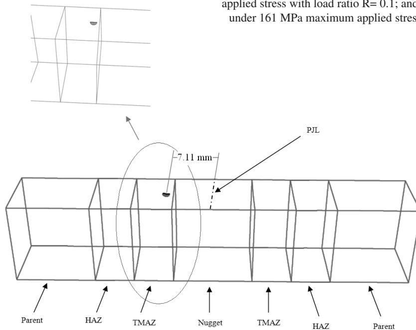
Fig. 3—Schematic image of initial crack location in developed model
