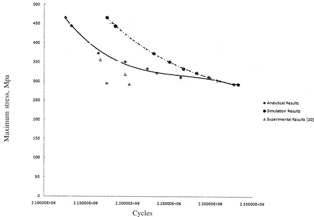
Fig. 10—Life prediction of Al 2024-T531 FSW joint
