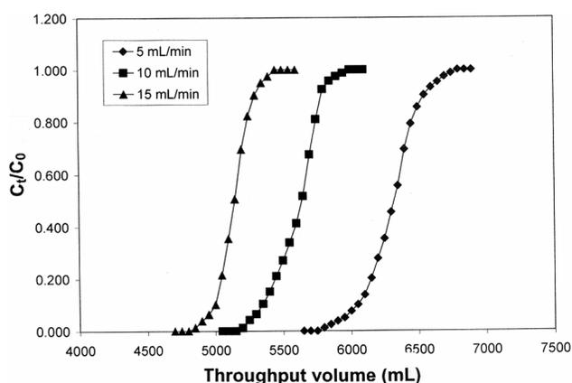
Fig. 8 — Effect of flow rate for the removal of Basic red 29 on EAAC column.
