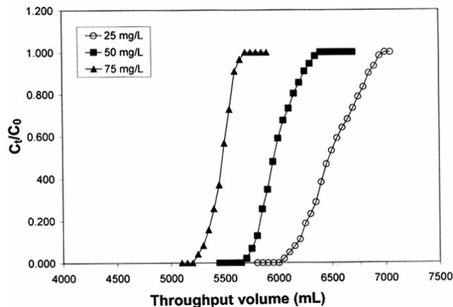
Fig. 3 — Effect of influent concentration for the removal of Acid blue 92 on EAAC column.
