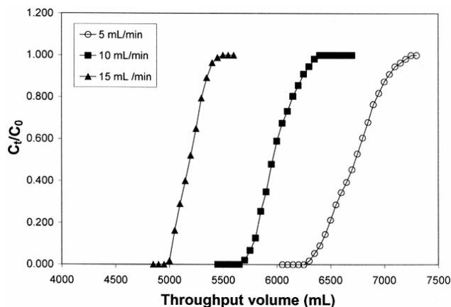
Fig. 7 — Effect of flow rate for the removal of Acid blue 92 on EAAC column.
