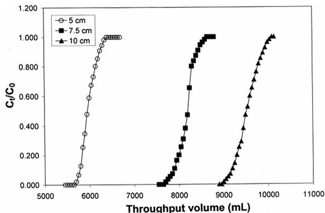
Fig. 5 — Effect of bed height for the removal of Acid blue 92 on EAAC column.
