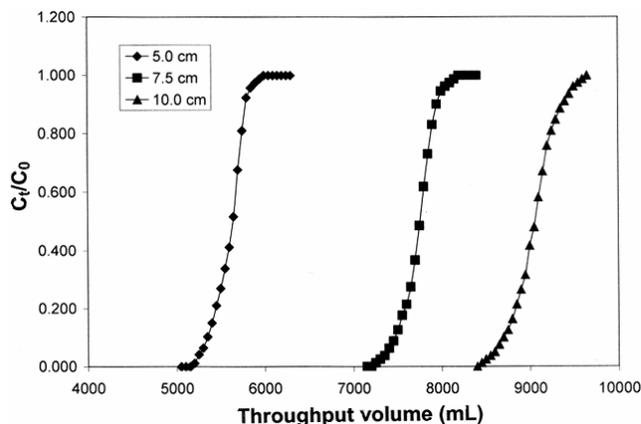
Fig. 6 — Effect of bed height for the removal of Basic red 29 on EAAC column.
