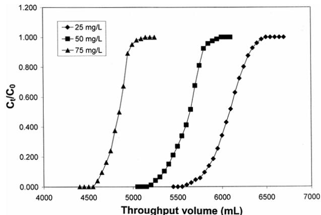
Fig. 4 — Effect of influent concentration for the removal of Basic red 29 on EAAC column.
