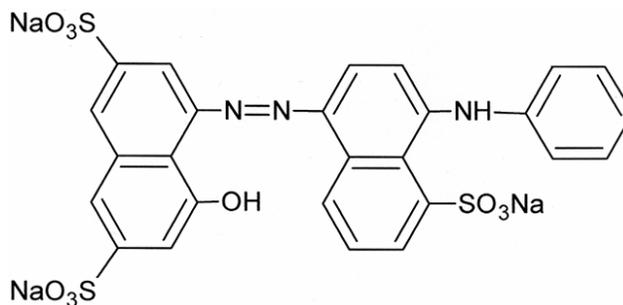
Fig. 1a — Structure of Acid blue 92.
