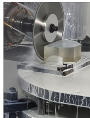
Schematic diagram shows steps involved in Stress Mirror Polishing. Photo shows polishing and Hex-cutting of a practice mirror blank — photocenterica, Bengaluru Credits: S. Sriram, IIA, ITCC
