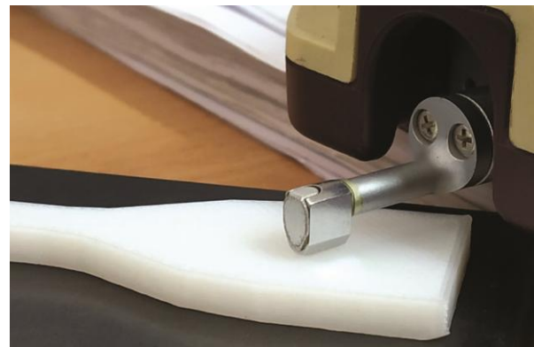
Fig. 6 — Surface roughness measurement setup.
