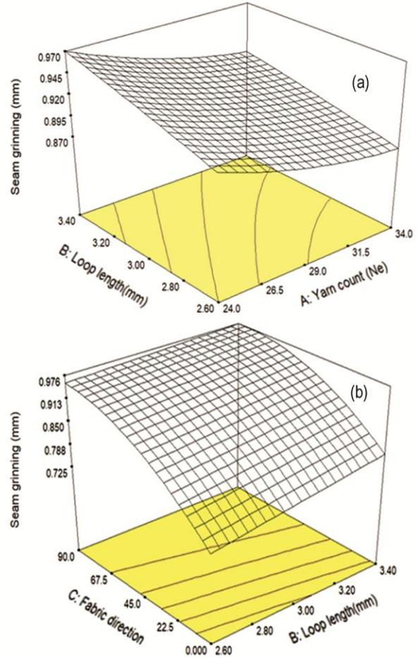
Fig. 6 —Effect of (a) yarn count & loop length and (b) fabric direction & loop length on seam grinning in cotton-lycra
