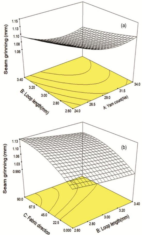
Fig. 4 — Effect of (a) yarn count & loop length and (b) fabric direction & loop length on seam grinning in polyester/cotton
