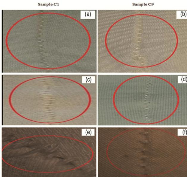
Fig. 1 — Seam separation during cyclic loading in samples C1 and C9 [(a) & (b) course, (c) & (d) wale and (e) & (f) bias directions]
