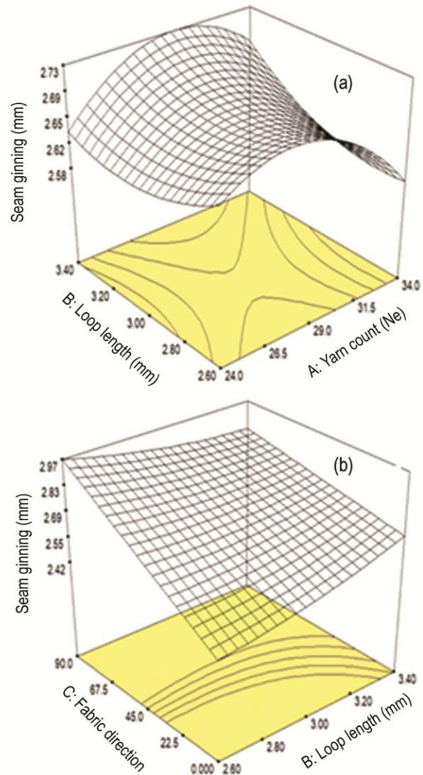
Fig. 3 — Effect of (a) yarn count & loop length and (b) fabric direction & loop length on seam grinning in 100% cotton fabric
