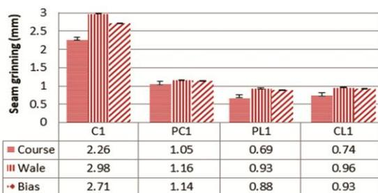
Fig. 2 — Effect of different fibres on seam grinning
