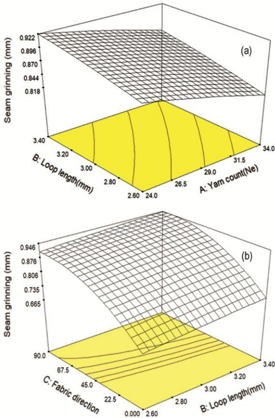
Fig. 5 — Effect of (a) yarn count & loop length and (b) fabric direction & loop length on seam grinning in polyester-lycra
