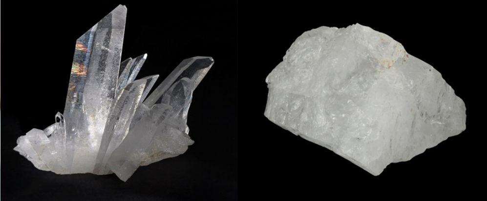
Quartz crystal (Crystalline solid) (left) and Quartz glass (Amorphous solid) (right) (Courtesy: Wikipedia and Enterprise Q)
