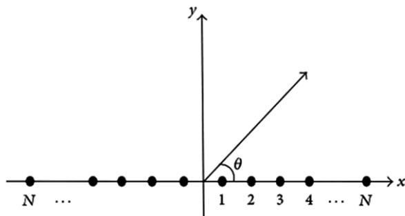
Fig. 1 — Geometry of linear array antenna
