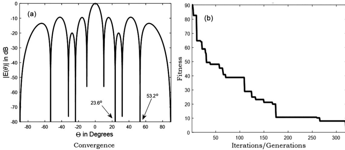
Fig.6 — (a) Radiation pattern with nulls at 23.6° & 53.2° with no constraint, (b) convergence plot
