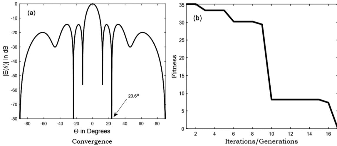
Fig. 4 — (a) Single null at  $23.6^\circ$  with no constraint, (b) convergence plot
