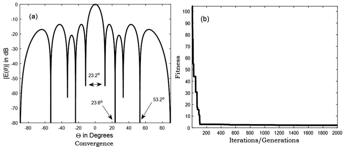
Fig. 7 — (a) SLL and BW Constrained null pattern @ 23.6° & 53.2°, (b) convergence plot
