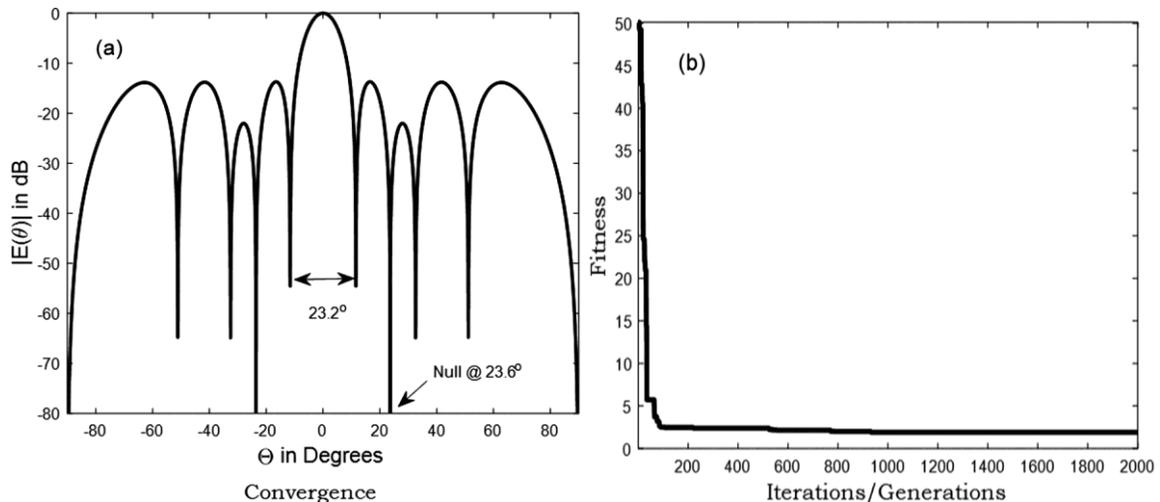
Fig. 5 — (a) SLL and BW Constrained null pattern @  $23.6^\circ$ , (b) Convergence plot
