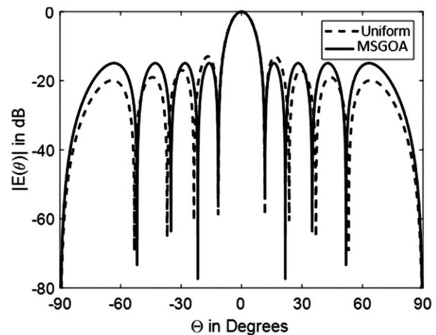
Fig. 2 — SLL optimised pattern with uniform BW constraint
