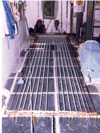
Fig. 2 Throw shuttle pit loom
