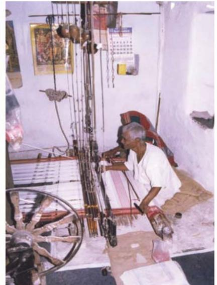
Fig. 3 Throw shuttle pit loom
