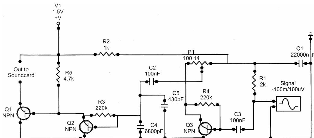
Fig. 2—Electronic diagram of the Amplifier/Filter
