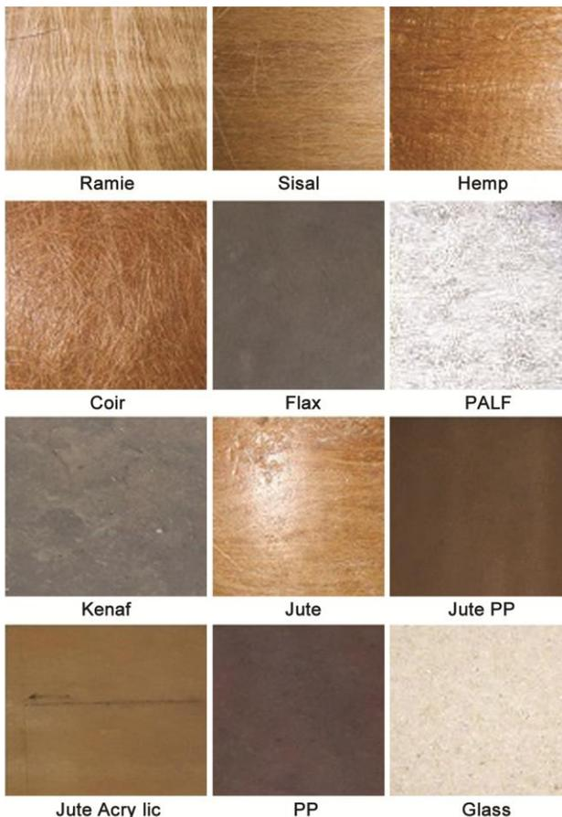
Fig. 5 — Surface photographs (top view) of natural fibre- polyester composites (in Nikon coolpix A 10 camera without magnification)
