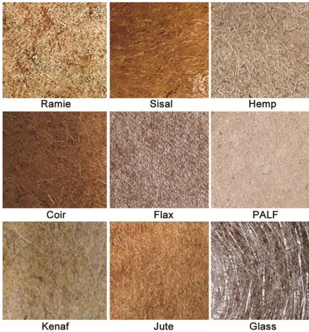
Fig. 4 — Surface photographs of nonwovens from natural fibres (in Nikon coolpix A 10 camera without magnification)
