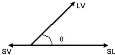
Fig. 2 — Balancing of forces for the equilibrium of liquid drop
