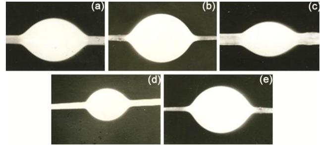
Fig. 3 — Liquid drops for contact angle measurement of (a) jute, (b) ramie, (c) flax, (d) sisal and (e) sunhemp
