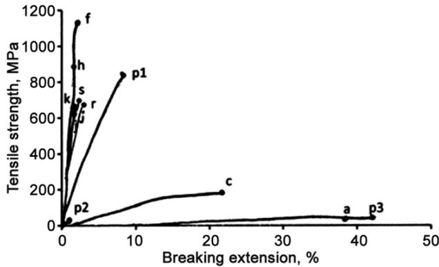
Fig. 1 — Strength-elongation curves of fibres and resin (r-ramie, s- sisal, h- sunhemp, c-coir, f-flax, p1 – pineapple, k- kenaf, j- jute, p3 – polypropylene, a- acrylic, p2 –polyester resin)
