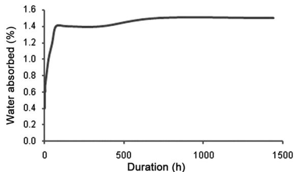
Fig. 6 — Water absorption of jute fibre composition
