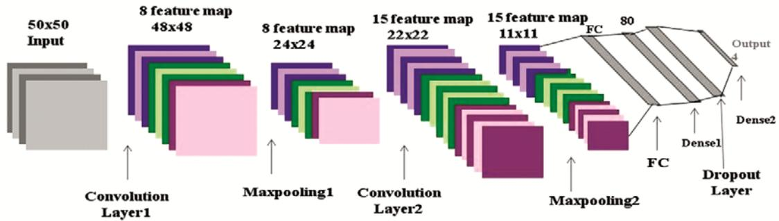
Fig. 2 — 2D-CNN architecture of type of diseases recognition
