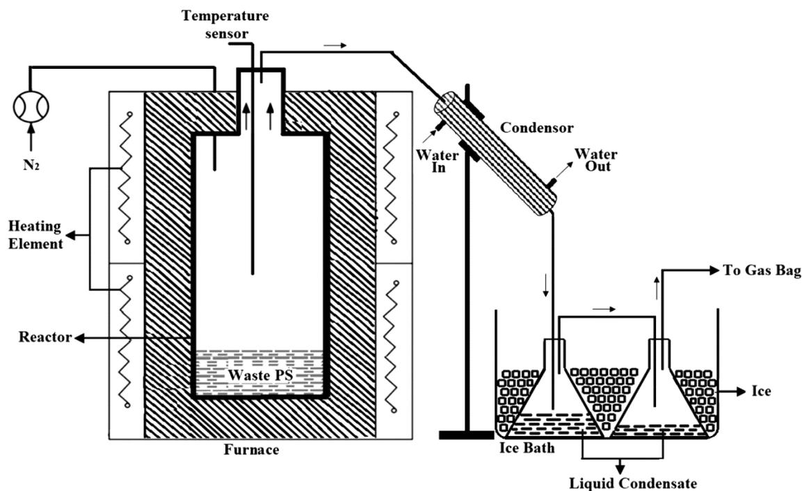
Fig. 2 — Schematic of experimental set up.
