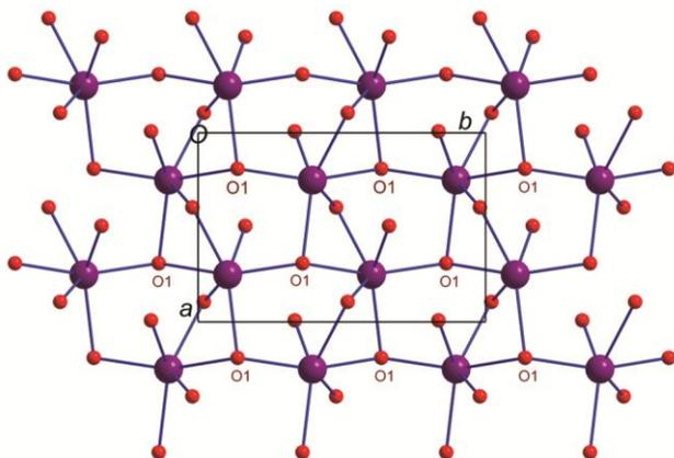
Fig. 8 — A portion of the 2D layer in  $\text{Tl}(\text{C}_8\text{H}_5\text{O}_4)$  showing hexacoordination around the central metal. O1 is a  $\mu_3$ -oxygen which binds to three  $\text{Tl}^+$  ions. For the interlinked  $\{\text{TlO}_6\}$  polyhedra see Fig. S11 in Supplementary Data
