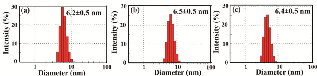
Fig. 5 — Hydrodynamic diameter (Size distribution histograms) of Triton X-100 based micellar structures (a) 1 mM Triton X-100 solution in water, (b) Triton X-100-Eu-C1-Pt-C2 adduct and (c) Triton X-100-Eu-C1-Pt-C2+TNP
