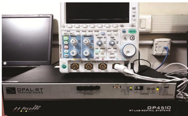
Fig. 11 — Setup of OPAL-RT: OP4510 real-time digital simulator.
