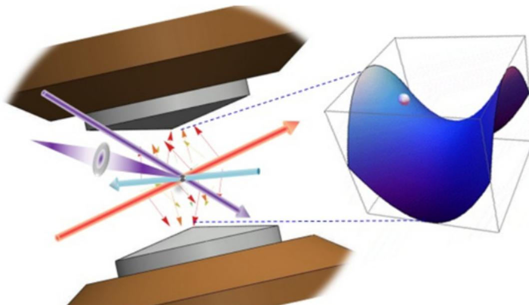
**Schematic of the single trapped ytterbium-ion confined in an electrodynamic potential created by an ion-trap. It requires five lasers for cooling the ion near the absolute zero temperature followed by probing its clock transition.**
