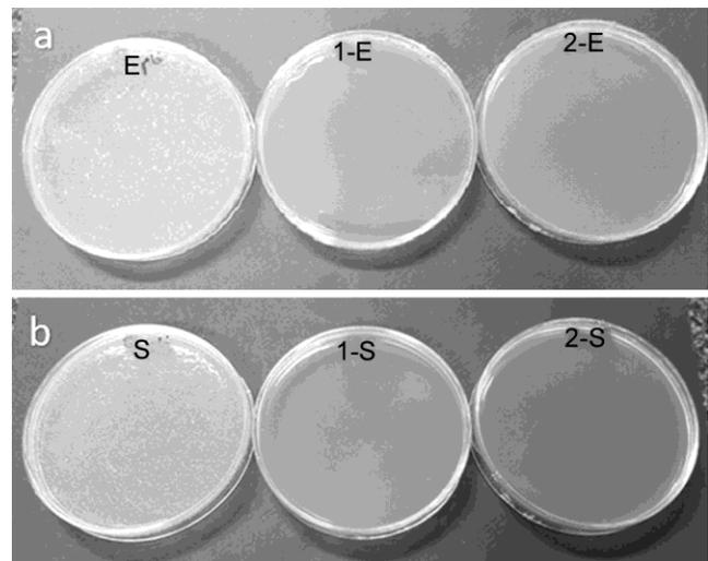
Fig. 2 — Antibacterial efficiency of control and treated fabrics (E) control, (1-E) compound 1, (2-E) compound 2 against *E. coli* (a); and (S) control, (1-S) compound 1, (2-S) compound 2 against *S.aureus* (b)
