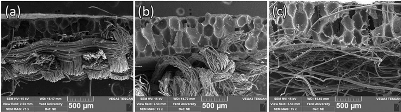
Fig. 5 — SEM images of fractured surfaces of the samples (a) WL, (b) KL and (c) NL
