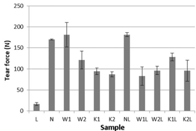
Fig. 3 — Average values of tear load for raw materials and synthetic leather samples
