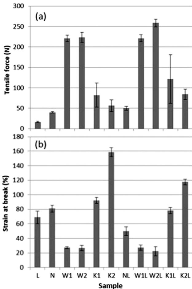
Fig. 2 — (a) Average values of tensile load and (b) strain at break for raw materials and synthetic leather samples
