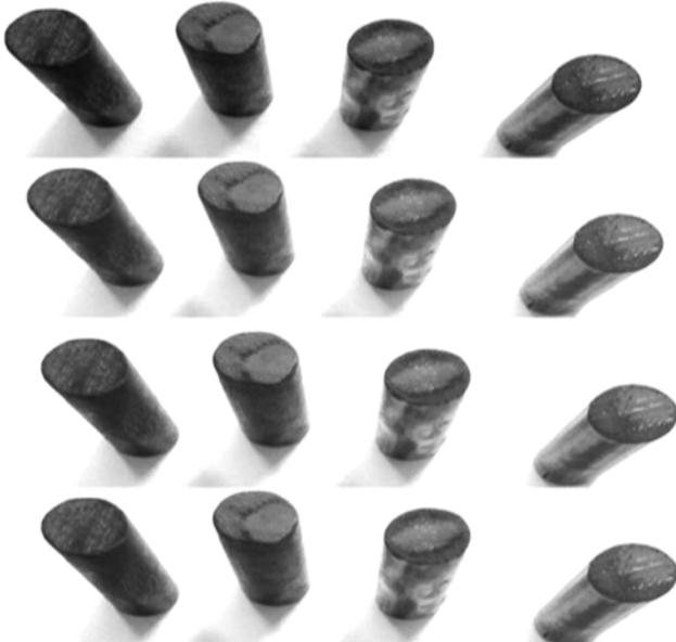
Fig. 7 — Worn surface of coated IN800 SGTBC.
