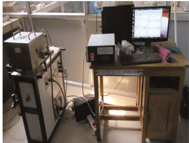
Fig. 5 (b) — Pin-on-disc test set-up with chamber heating.
