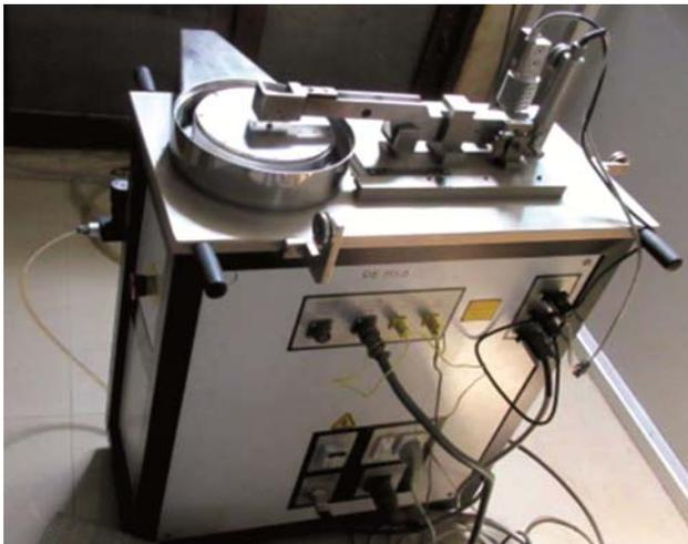
Fig. 5 (a) — Pin-on-disc test set-up.
