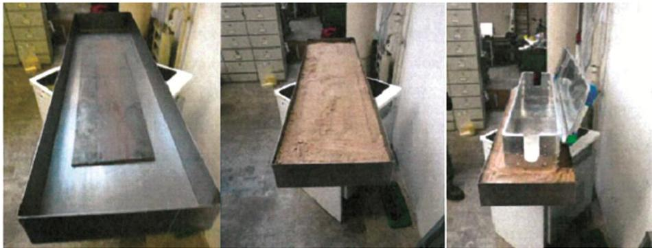
Fig. 2 — Building stage of corrosion cell.
