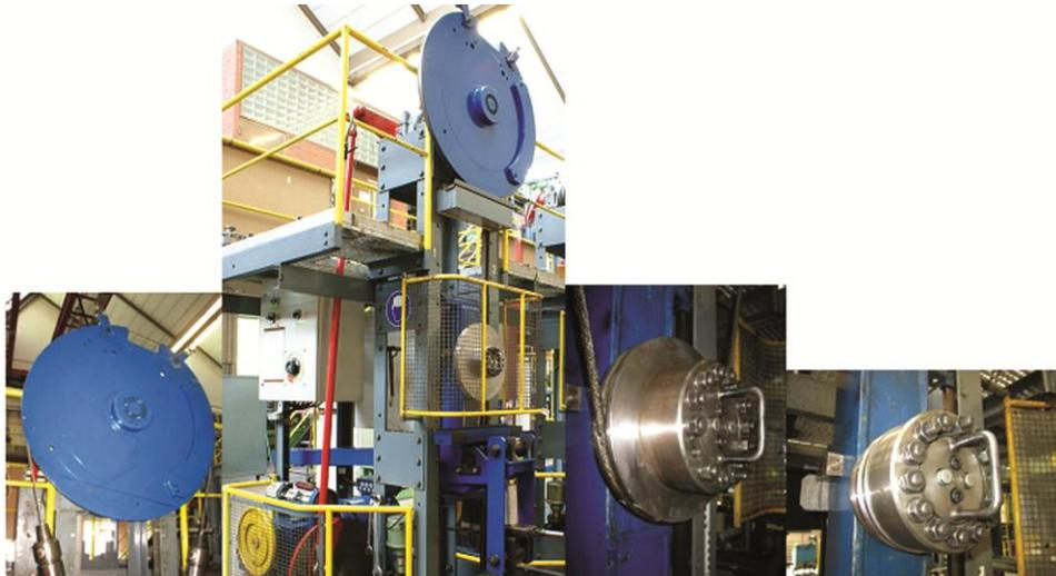
Fig. 5 — Test machine for bending fatigue.
