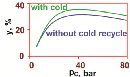
Fig. 6 – Cold recycle effect on liquefier yield
