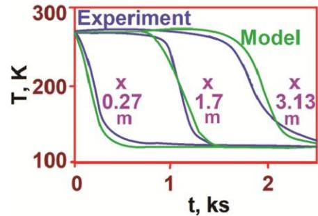
Fig. 3 – HGCS validation - T versus t for varying x
